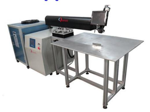
Questt Laser welding machine - Professional solution to the manufacture of Channel letter to make sidewalls and face or sidewalls and backwalls together.
